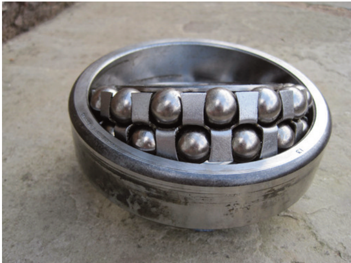
10th bearing opened up showing double row of balls. You can just see the wear at the back of the casing
