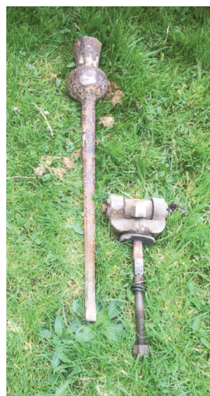
The broken clapper at Broadhembury
